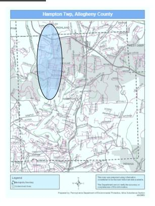
plant is treating drainage from the closed Wildwood Coal Mine (Willow Run in circle on map of Hampton Township showing mine transecting the township, right.) A sewer line is also in place in the stream channel.
